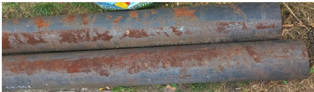
Figure 5. Metal tubes used to simulate the load due to street traffic
