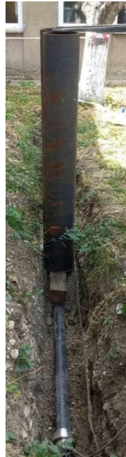
Figure 12. Applying an external load (122.3963 kg) to the defect area to simulate localized traffic overload
