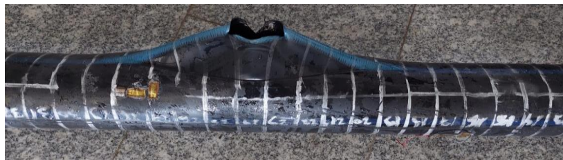
Figure 18. PE100 polyethylene pipe failure evaluated under multiple stress conditions
