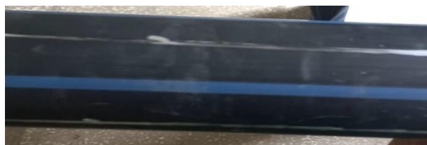
Figure 3. The PE100 polyethylene pipe used for the multiple stress test
