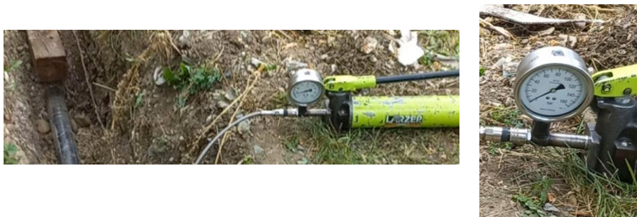
a) b) Figure 6. The Rems Push manual pressure test pump: a) general view; b) detail
