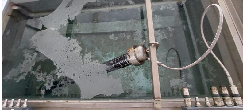
Figure 14. Internal pressure testing of the pipe
