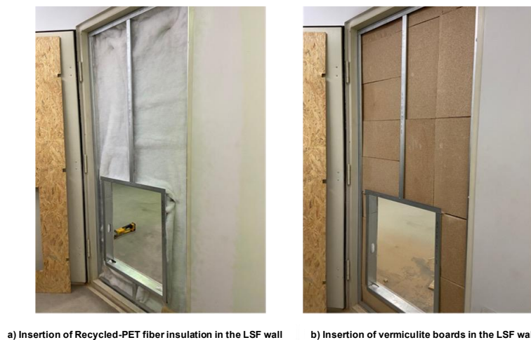
Figure 3. Different configurations of the test wall. a) Wall with PET wool blanket; b) wall with vermiculite boards.Source: Prepared by the authors, 2024.
