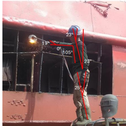
Figure 2. Posture of worker 2 in the cutting section
