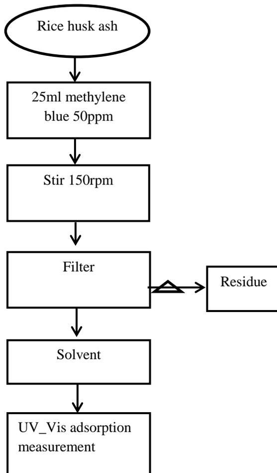
**Diagram 1.** The experimental procedure to investigate the influence of pH, rice husk ash mass and adsorption time to the MB adsorption capacity of rice husk ash
