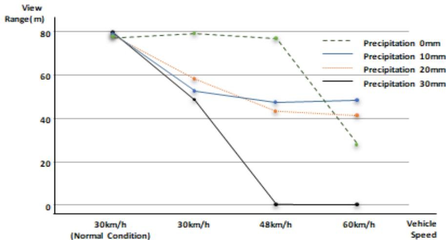
Figure 4 ADAS data variation depending on vehicle speed
