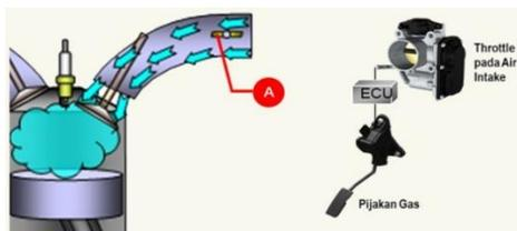
**Figure 1.** *Throttle by wire*
