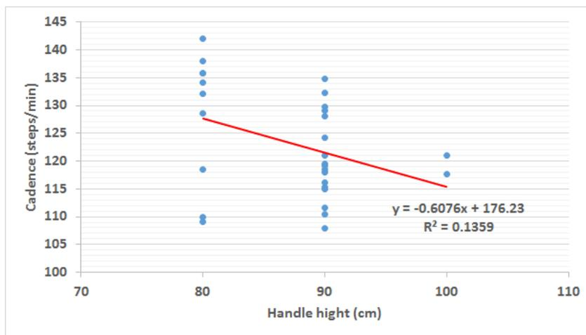
Figure 7 Scatter plot on Cadence-stair handrail height
