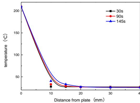
Fig4.axial temperature distribution of outer wall of pipe at different heating times
