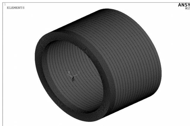
Fig2. meshing the geometric model
