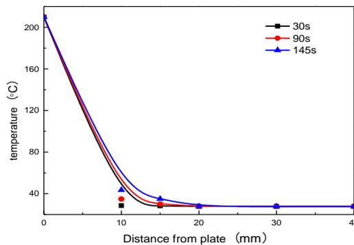
Fig5.axial temperature distribution of pipe wall at different heating times
