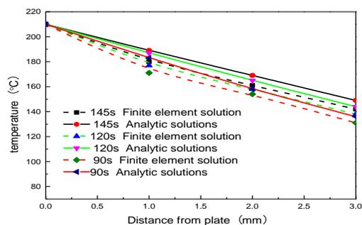
Fig6. Comparison of temperature distribution between finite element solution and analytic solution at different heating time
